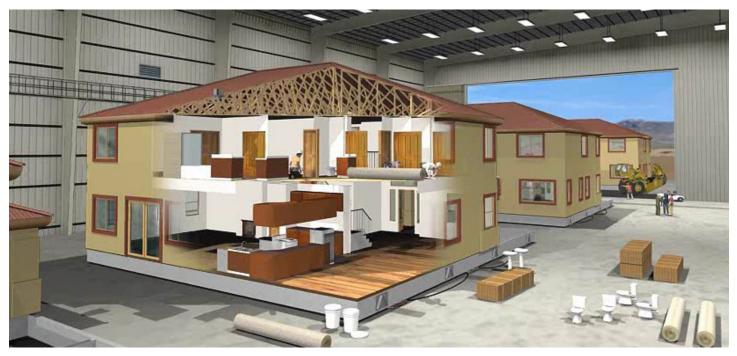
The Nubuild Whole House Factory comprises 16 work stations. Starting with the foundation, the house moves along the assembly line, stopping for two hours at each station. The Nubuild factory can produce a complete 1,000 s.f. to 5,000 s.f. home in 32 hours. The average production home in the U.S. takes over 120 days to build.
