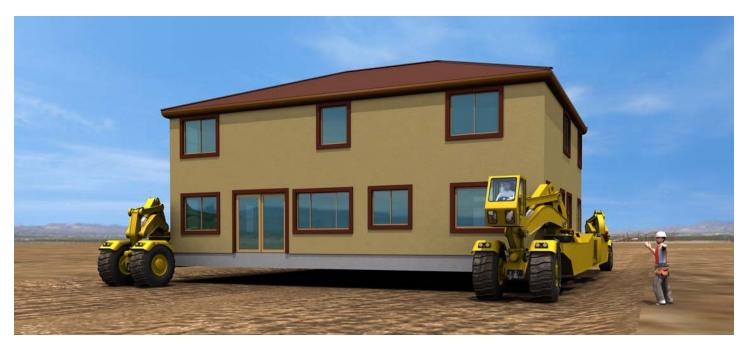
The Rhodemaster is comprised of twin Rhodesters. The Rhodesters are synchronized and operate in unison to lift a complete 1,000-square-foot to 5,000 square-foot home by its foundation. The Rhodemaster then drives the home to its assigned lot, using GPS coordinates to set the home in its correct location within the community development.
